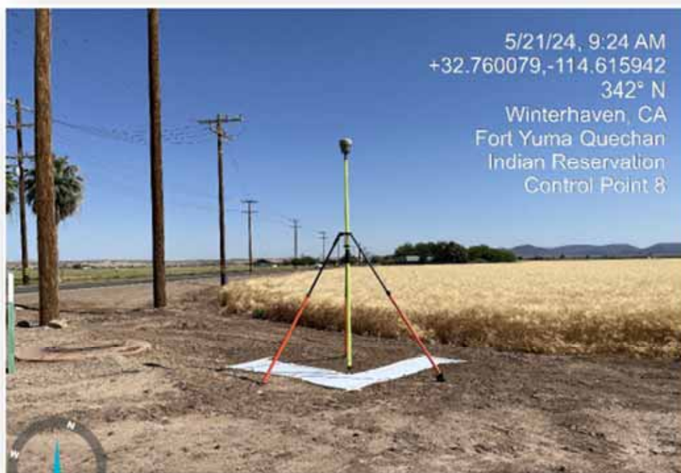
Figure 13. GLA-KNB LiDAR survey ground control point
