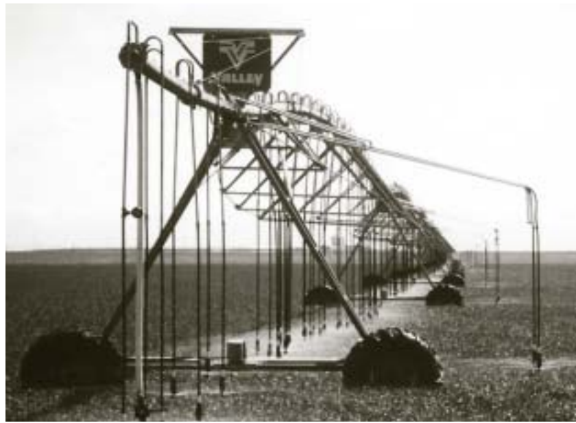
Western’s Energy Services program has promoted energy- and water-saving techniques like low energy precision application, or LEPA, which allows irrigators to place water where it’s needed. The technique reduces evaporation, thereby reducing water and energy consumption. This field is in eastern Colorado.
